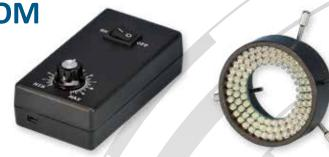
side 35 mm. The LED ring light is mounted with three screws on an adapter, which is screwed on to the zoom. Scope of delivery includes a power pack with infinitely variable dimming.
