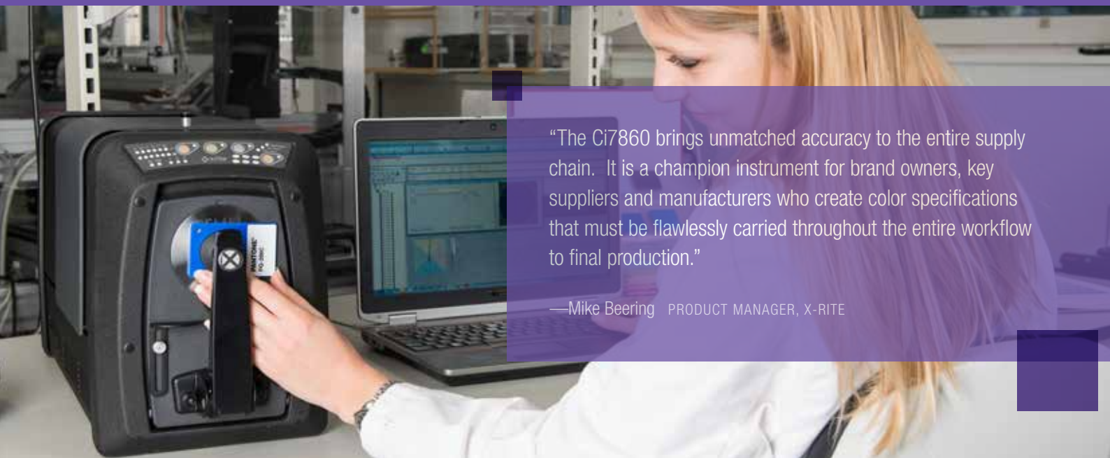
▲ PICTURED: Ci7860 benchtop spectrophotometer measuring a PANTONE plastic standard in a lab
